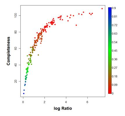
Bubble chart of the relationship between log(Ratio) and completeness, being the color gradient the slope value.
